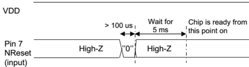
Figure 43. Manual Reset Timing Diagram
