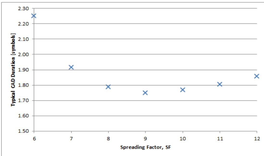
Figure 12. CAD Time as a Function of Spreading Factor
