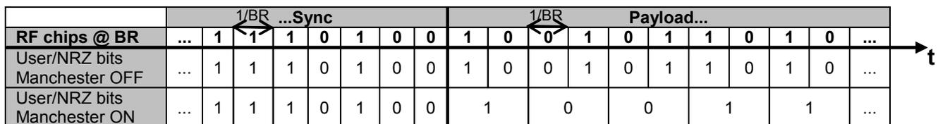
Figure 36. Manchester Encoding/Decoding
