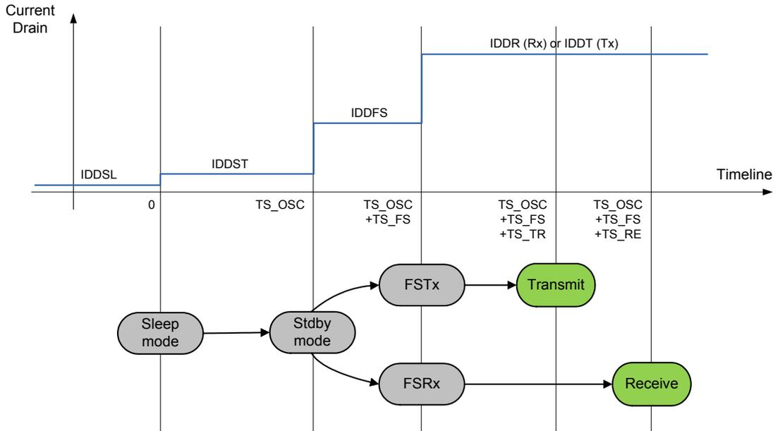
Figure 17. Startup Process
