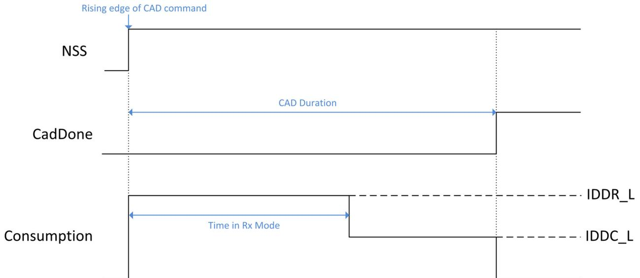
*Figure 13. Consumption Profile of the LoRa CAD Process*
