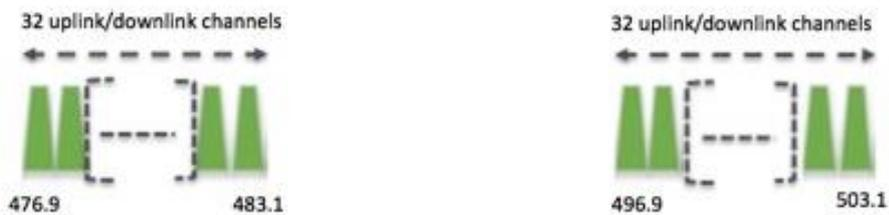
Table 43: channel plan type B for 20MHz antenna channel frequencies
