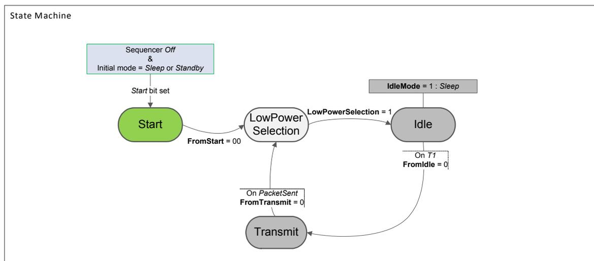
Figure 53. Beacon Mode State Machine
