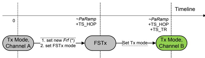
Figure 22. Transmitter Hopping
