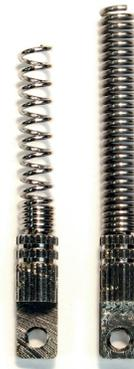
Figure 3: 916MHz (L) and 315MHz (R) Helical Antennas
