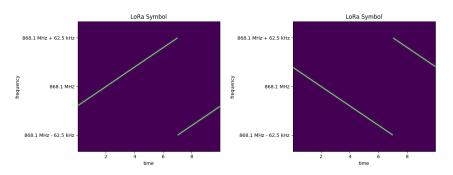
Time of frequency jump determines which data is encoded
