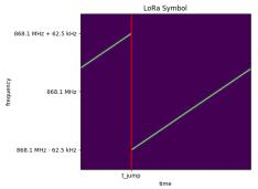
Time of frequency jump determines which data is encoded
