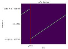
Time of frequency jump determines which data is encoded
